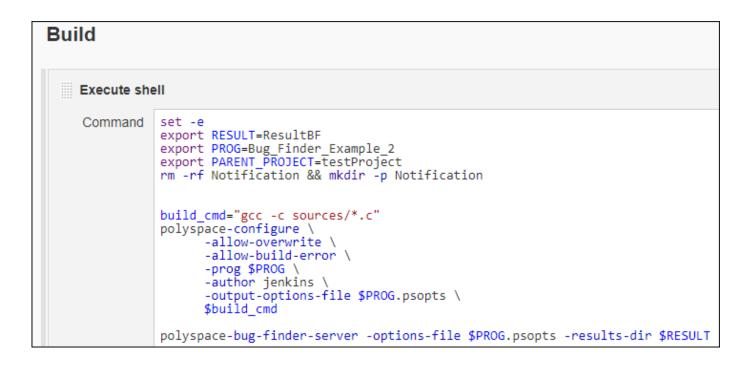
The scripts run a Polyspace analysis and upload results to the Polyspace Access web interface.
